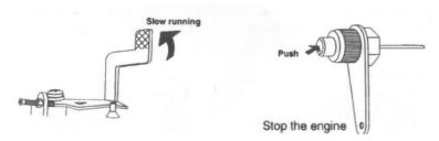
Stopping the sprayer after completing spraying:
