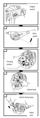
When the engine has started, return the choke lever gradually to the fully opened
